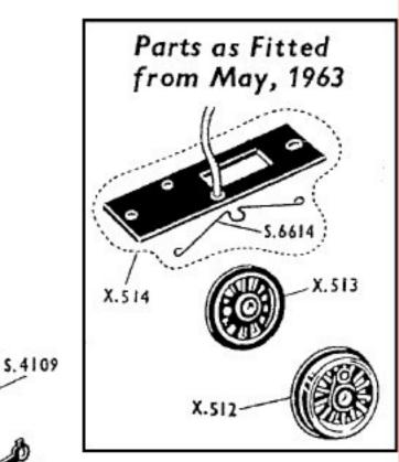
NOTE: Locomotive R.252 may be modified to operate from overhead power stupply by fitting Pantograph X.176 and replacing T.V. Suppressor X.224 by Switch Assembly X.180. Replacement of Body R.252/1 by R.254/1 is not essential but is recommended as the latter bears the printed switch position indications.
